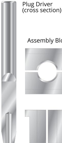
Electroline's swagless rope terminations can be quickly installed in the field without the need for expensive tools, chemicals, pressure, or heat. Using an assembly kit can speed up the installation process. The assembly block helps prevent damage to the rope and the plug driver can help seat the plug as well as assist with flaring the rope strands. Electroline's assembly instructions demonstrate how to use the assembly kit when terminating a rope.
