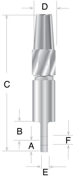
Electroline synthetic rope fittings for Kevlar ropes with extruded jackets excel in meeting the need for a quick, reliable end termination. The fittings perform on polyurethane, Nylon II, and Hytrel jacket materials for ropes with the following construction: standard wire rope, contra-helical, parallel, and electro-mechanical. This fitting features a clevis (fork/jaw) connection and a swageless rope termination, allowing it to be quickly installed in the field without special tools.
