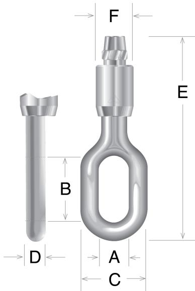
Electroline's towing eye fitting features a swageless rope termination, allowing it to be quickly installed in the field without special tools or processes.
