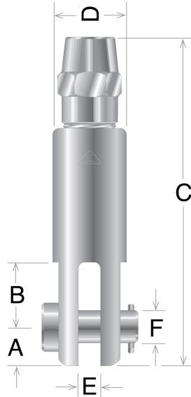
Electroline synthetic rope fittings for Kernmantle rope are supplied with the SAR1000 series internal plug. The sleeve has no exposed thread when assembled and is retained in the socket with a set screw. This fitting features a clevis (fork/jaw) with an included pin. The swageless termination allows it to be installed in the field without special tools or processes.
