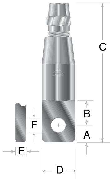
Electroline synthetic rope fittings for Kernmantle rope are supplied with the SAR1000 series internal plug. The sleeve has no exposed thread when assembled and is retained in the socket with a set screw. This fitting features an eye fitting and a swageless termination, allowing it to be installed in the field without special tools or processes.
