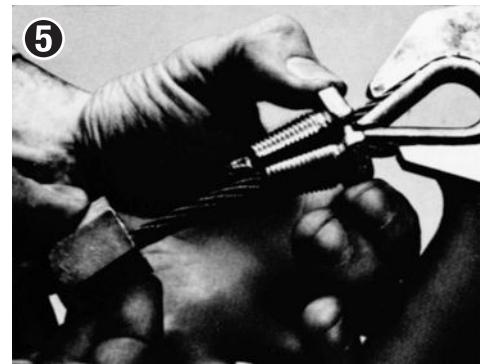
**STEP 6:** Grip the opposing parallel flats of the two clamp halves in vise as shown, and then brush the exposed threads liberally with a high-viscosity lubricating oil (or paste like Lubriplate). Too much is better than not enough - and *do not omit this step*.
