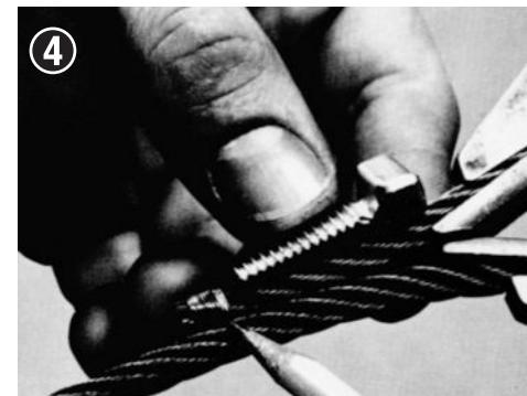
**STEP 5:** With your fingers, turn the Safe-Line Nut onto both threaded halves for a thread or two - taking care that the alignment of both halves is correct and no cross threading occurs.
